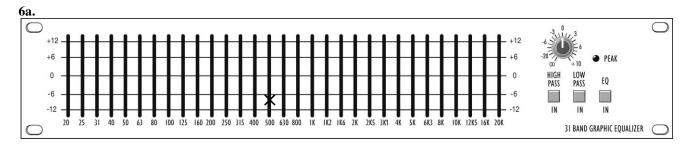
A mark at 6 dB below 0 on the 500 Hz fader. All other faders should have been at 0.
