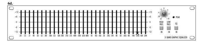
A mark at 12 dB below 0 on the 12.5 kHz fader. All other faders should have been at 0.
