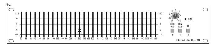
A mark at 6 dB below 0 on the 400 Hz fader. All other faders should have been at 0.
