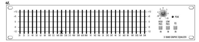
A mark at 12 dB below 0 on the 200 Hz fader. All other faders should have been at 0.
