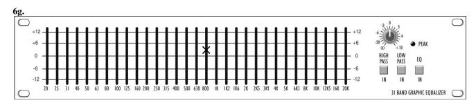
A mark at 3 dB above 0 on the 800 Hz fader. All other faders should have been at 0.
