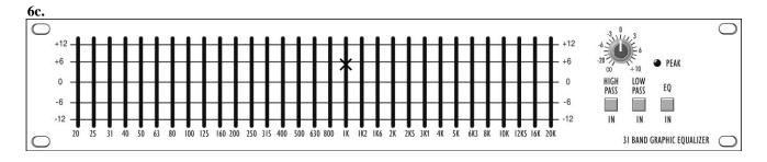
A mark at 6 dB above 0 on the 1 K fader. All other faders should have been at 0.
