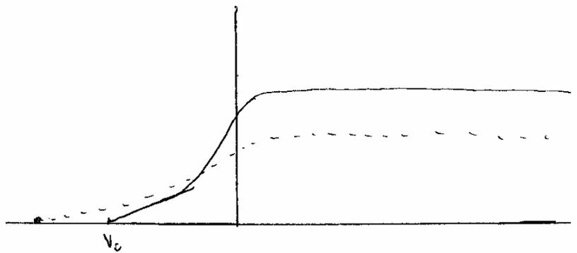
Most students sketched a curve with a lower maximum current as expected, but not many showed the cut-off potential to the left of  $V_0$ .
