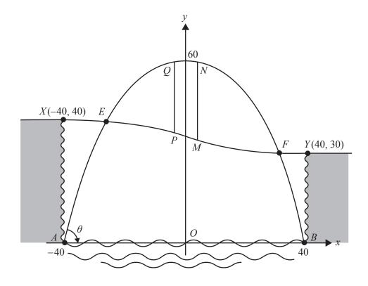
The main frame of the bridge has the shape of a parabola. The parabolic frame is modelled by  $y = 60 - \frac{3}{80}x^2$  and is connected to concrete pads at B(40, 0) and A(-40, 0).
