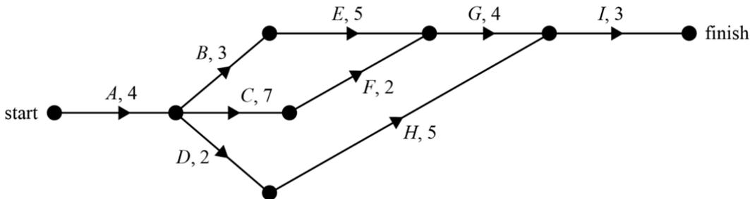
By sketching the network as shown above or following the table of predecessors, three paths are possible from the start of activity A to the finish of activity I.
