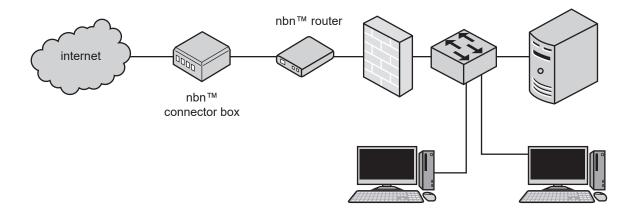
A small office network connects to the internet via the National Broadband Network (nbn<sup>TM</sup>), as shown in the diagram above. One morning, no computers on the network could access the internet. When the network connection on one of the computers was checked, the network cable was found plugged in and the nbn<sup>TM</sup> router indicator light was on.
