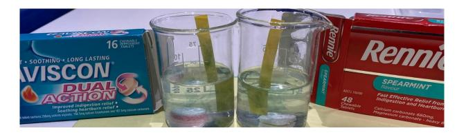
Experimental set-up for the testing of two commercial antacid tablets using universal indicator paper.
