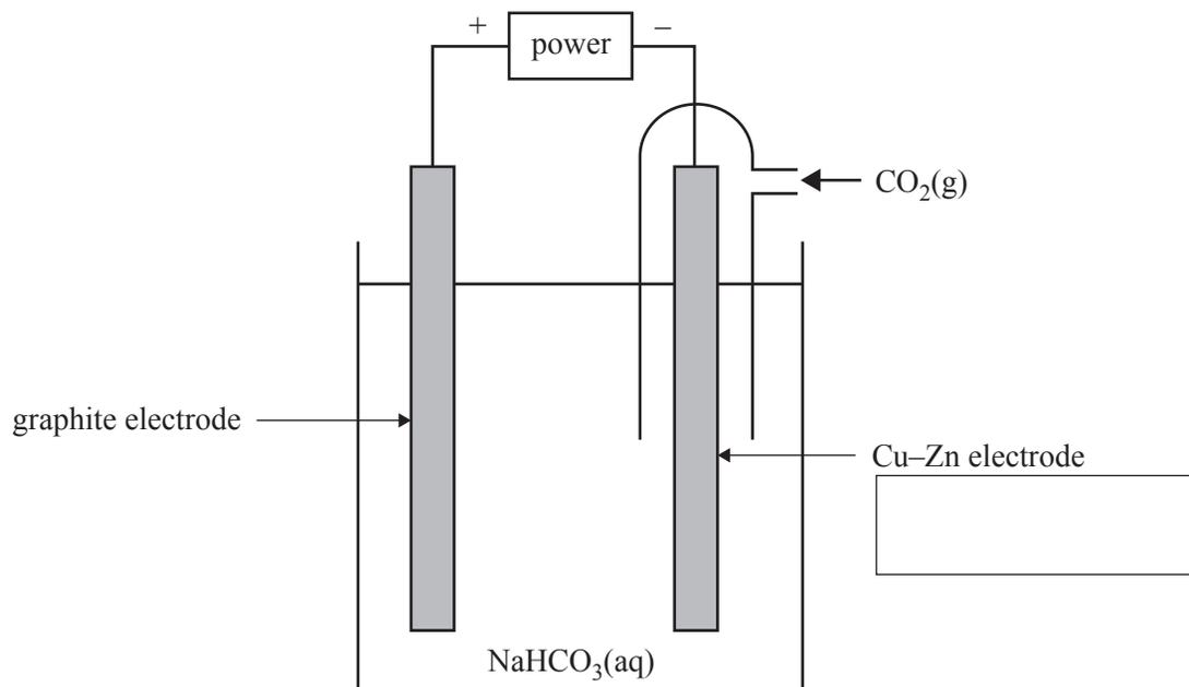
The following half-cell reactions occur in the  $\text{CO}_2$ - $\text{H}_2\text{O}$  electrolysis cell.
