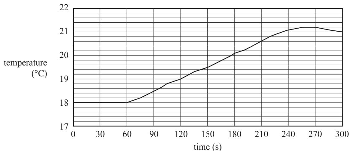
The calorimeter was calibrated using a current of 2.7 A, starting at 60 s. The current was applied for 180 s and the applied voltage was 5.4 V.
