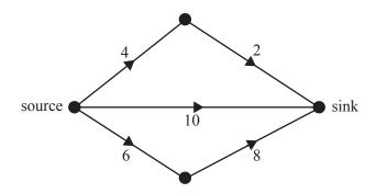
The maximum flow, in litres per minute, from the source to the sink is
