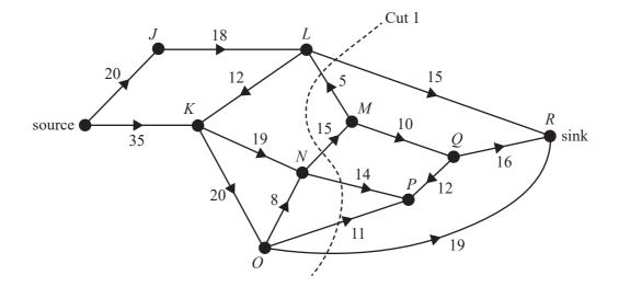
When considering the possible flow of stormwater through this network, many different cuts can be made.
