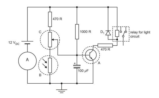
Connecting the ammeter in parallel was a common error.
