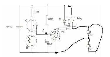
Many students did not know the difference between series and parallel circuits. The lights are 12 V and there is a 12 V supply, so the inference is that the lights are in parallel.
