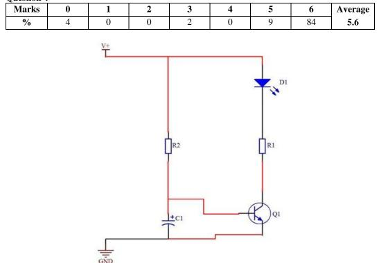
The majority of students answered this question correctly. Some students were not sure how to connect the base of the transistor to the capacitor; they drew a line to the middle of the capacitor symbol.
