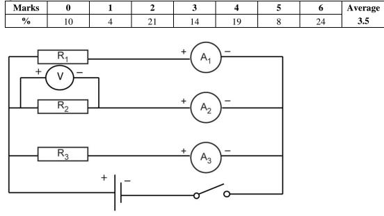
The voltmeter could be connected differently, as long as it reads the voltage of R<sub>2</sub>.
