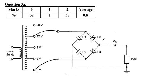
This question required students to make some rough determinations about the stated RMS voltages on the multiple tapped transformer when converted to the possible peak voltages. Both the 0 V and the 12 V tap had to be connected to the bridge rectifier. The following mathematical solution proves the 0 V and 12 V connections are correct.
