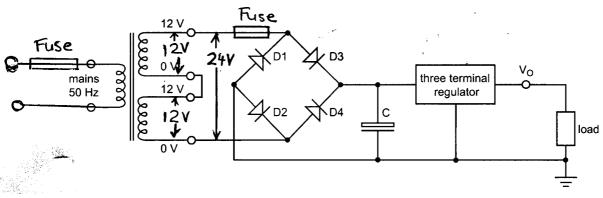
It was acceptable to place a fuse in either the primary or secondary part of the transformer.
